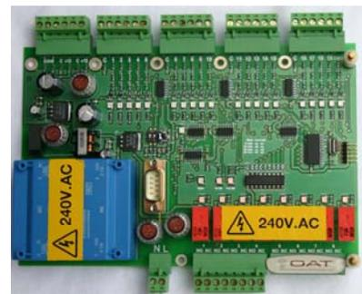
The system is designed to be fail safe such that should the controller, receiver or one of the sensors fail, the lighting for that floor will turn on. A commissioning mode allows quick set up and testing of the system
